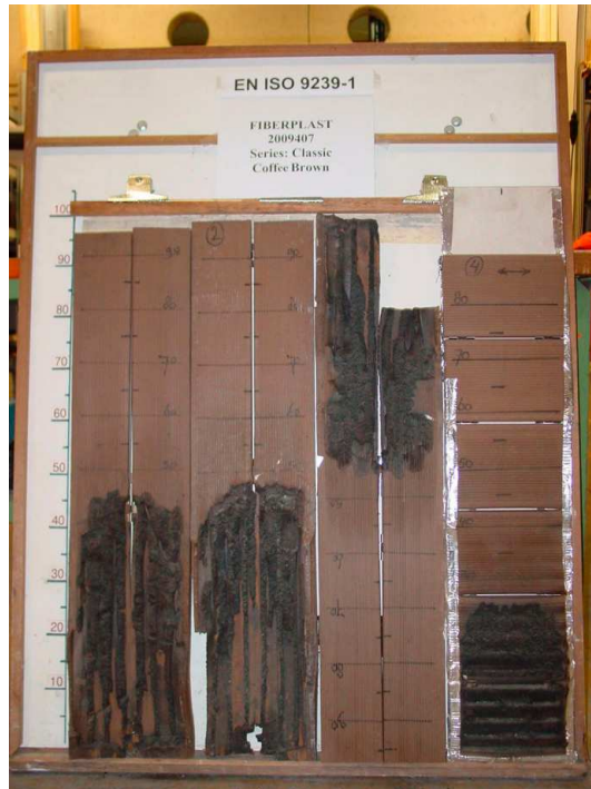
Specimens type Coffee Brown after testing
