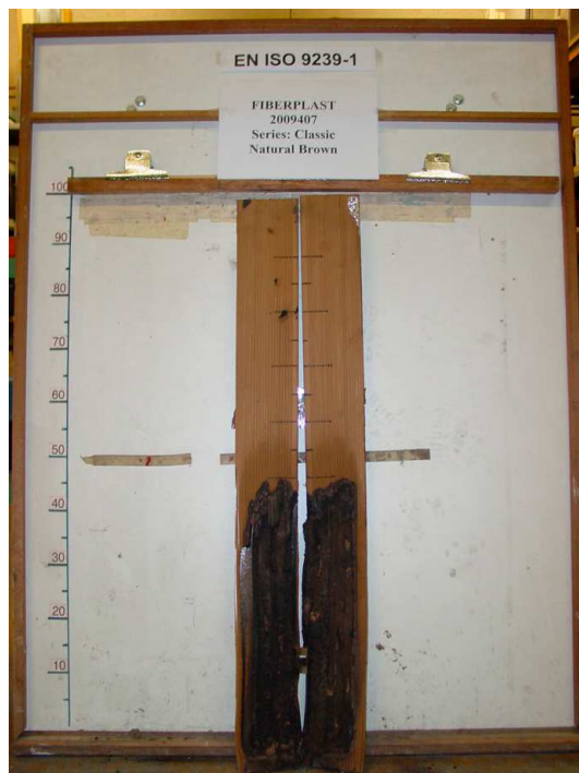
Specimens type Natural Brown after testing
